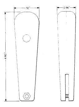
A two-piece plastic handle arranged to accommodate a No. 788 type tool for use on No. 88 type connecting blocks.
