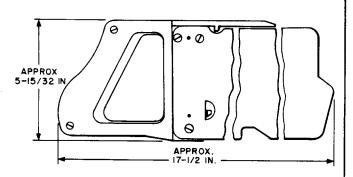
For use in bulk handling of 200A blanks and coded cards when servicing 1A-type translators.
