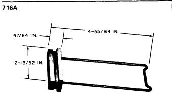
Ratchet head. This tool forms part of 1014B tool kit. For use in conjunction with 715A tool when replacing coils of AF-, AG-, and AJ-type relays.
