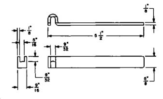
Guide holder. For use in adjusting 1-type guides.
