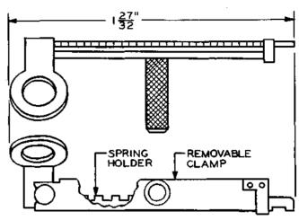
Spring holder and removable clamp. For use in holding movable make contact springs in positions 1 through 12 on AF-, AG-, and AJ-type relays during removal of the card from the relay.
