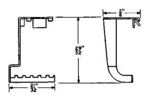
Spring holder. For use in holding the upper group of movable break contact springs on AF-, AG- and AJ-type relays during removal of the card from the relay.
