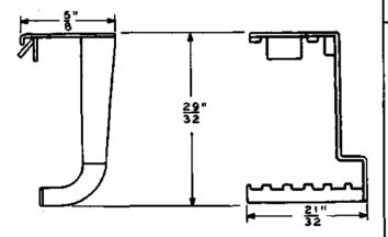
Spring holder. For use in holding the lower group of movable break contact springs on AF-, AG- and AJ-type relays during removal of the card from the relay.
