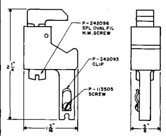
Cord holding detail. Replaces cord holding detail R-1648, detail 2. For use on vertical drive shafts.
