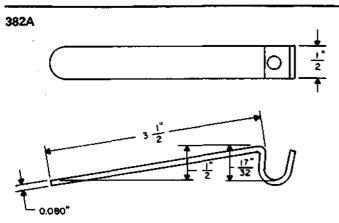
Trip rod holder. For use on 4- and 14-type trip rods.
