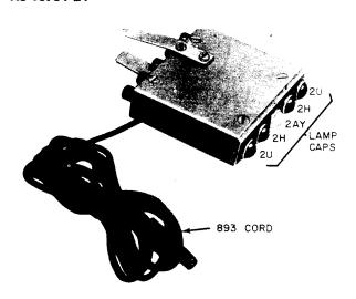
Consists of a molded case enclosing five 2Y lamps equipped with individual connectors and a common battery lead. Optional clip not furnished but may be ordered separately. For use in No. 5 Crossbar System to indicate closed contacts of 293-type relays.
