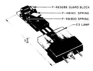
Contact closure indicator. This tool forms part of the J94724 contact closure test set. For use on 280- and similar-type relays.
