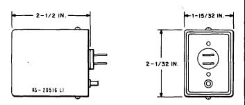
A metal enclosed, single-unit device consisting of a relay driven by a transistorized, astable multivibrator which is powered off a 48-volt dc source. Intended to provide ground pulses for rotating the number wheels of from one to three 14-type message registers at approximately 5 Hz to facilitate cleaning of the registers with a vacuum cleaner.
