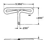
Used to release the housing and door locking mechanisms of the No. 1A type coin telephone sets after first opening the locks with keys.
