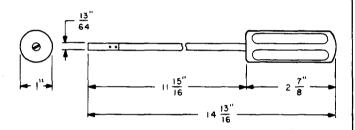
Sleeve terminal locking tool. For use on 49-type jacks to twist the sleeve terminal to lock the sleeve in position.
