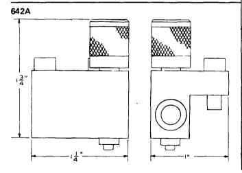
Dial locking tool. Replaces the D-178352 tool. For use as a dial lock on the KS-13835 readers in AMA Systems while adjustments are being made.
