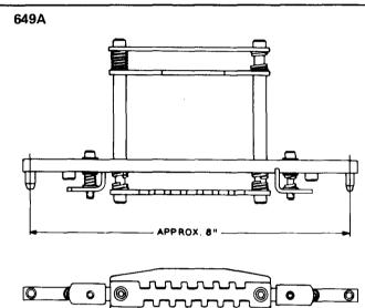
Pin locking tool. Replaces the D-178386 tool. For securing the perforator pins on a KS-13882 perforator during shipment in the KS-14131 carrying case.
