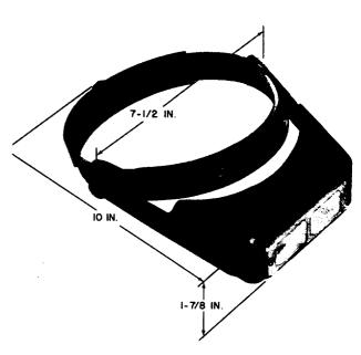
A binocular magnifier consisting of an adjustable headband and a shaded plastic visor equipped with a replaceable lens plate. Visor is hinged to headband for easy eye level adjustment. Magnifier has magnification of 2-1/2 power at 8-inch focal length. For use in adjusting miniature wire spring type relays.
