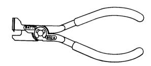
Used for attaching individual wires to the 711 connector mandrel.
