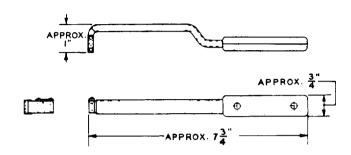
Commutator brush guide mounting tool. For use in installing rear guides on panel commutator brushes.
