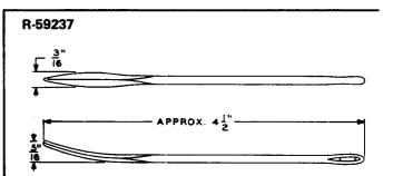
Sack needle. Steel needle for use in sewing cable forms (PBX installation only).
