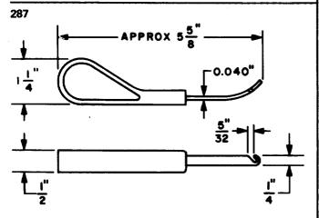
Curved cable sewing needle. For use in sewing local cable (PBX installation only).
