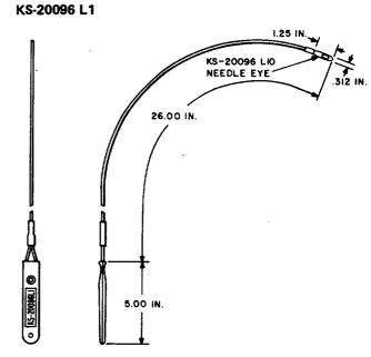
A curved, insulated, metal rod equipped with an insulated eye at one end arranged to thread four 22-gauge insulated wires. The other end is provided with an insulated handle. The KS-20096 L10 needle eye may be ordered as a separate item to replace damaged eyes on KS-20096 L1 needles in the field. For use in running jumpers on the No. 1 ESS main distributing frame.
