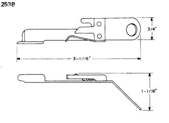
Brake plate. Replaces the 253 tool. For use on Aand B-type sequence switches.
