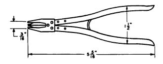
For use in installing external snap rings in the 1-type translators.
