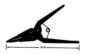
For use in replacing rings of Dzus fasteners.
