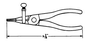
For use in installing internal snap rings in the 1-type translators.
