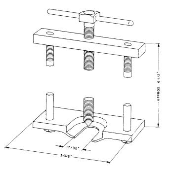
**Bearing puller.** For replacing bearings in KS-7664 and KS-7781 controllers.
