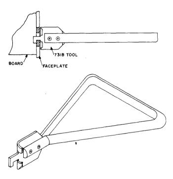
**Card puller.** For use in extracting packages in the switch unit or control unit. For use in the No. 1 ESS.
