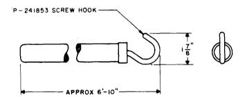
**Cross-connection wire puller**. For use in pulling cross-connection wires through distributing frames.
