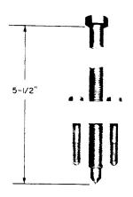
Gear and pulley puller. For use with Owatonna Tool Company 950 bearing pulling attachment to remove ball bearing race from shaft of blower motor of the KS-16001 dehydrator.
