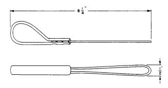
Wire loop puller. For use in sewing cable (PBX installation only). Can also be used as a replacement for the 291 tool for use on terminal block fanning strips which was rated Mfr Disc.
