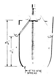
**Bearing Puller.** Also see bearing pulling attachment. For general use.
