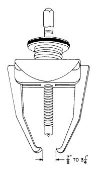
Gear puller. For use in removing a gear from indexing assembly of the 1A card writing unit.
