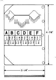
Perforated metal plate. For use in visually translating coded perforations in AMA tape.
