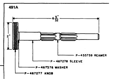
Forms part of the 1000A tool kit. For use in replacing bushings on reciprocating bar-type interrupters.
