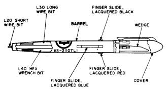
Consists of a brass, double-ended, pen-type combination tool containing three retractable bits at one end and a wedge-shaped extension at the other end.
