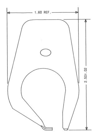
Fig. 6—AT-8927 C Bridge Removal Tool—Front View
