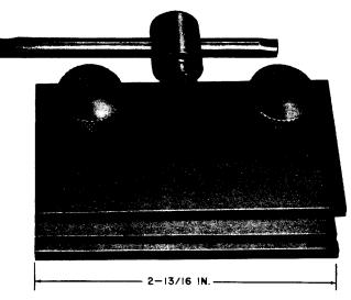
Core plate replacer. Replaces the 716C tool. Forms a part of the 1014B tool kit.
