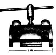
Core plate replacer. Order this tool for replacement purposes only if the office is equipped with the 1012A tool kit. The 1012A tool kit is no longer available as a complete kit. For use in replacing core plates of 286-, 287-, and 288-type relays.
