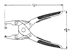
Pawl pin replacer. Forms part of the 1001A tool kit. For use in replacing pawl pins on 197- and 198-type switches.
