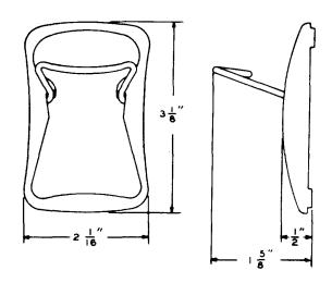
Folding soldering copper rest. For use in supporting KS-8740 soldering coppers for PBX installations only. Use of this tool with the KS-14440 soldering copper is optional when the 504A tool is not provided.
