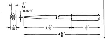
A 3-1/8 inch screwdriver. Replacement part for the 72 tool. For use on reciprocating bar-type interrupters and connecting blocks.
