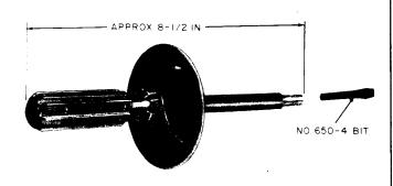
Equipped with 650-4 bit only. A torque screwdriver having a capacity of 12 inch-pounds. For use in tightening mounting screws of wire spring type relays equipped with P-19A890 flexible mountings.
