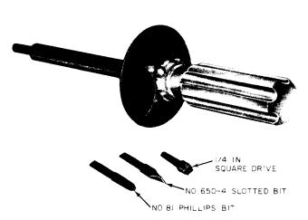
A torque screwdriver having a capacity of 50 inch-pounds. For use in tightening recording head mounting screws and capstan mounting plate screws on the KS-19125 L3, KS-19647, and KS-19829 recorders.
