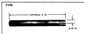
Coil setter. Replaces the 717A tool. Forms part of 1014B tool kit. For use in replacing coils of AF-, AG-, AJ-, AK-, 286-, 287-, and 288-type relays.
