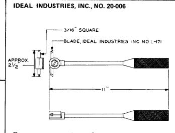
For use on generator and motor commutators and on interrupter drums.
