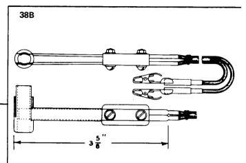
Consists of a 38A lamp socket equipped with an M2CP cord (6' 6''). Intended for use with a 2-type switchboard lamp. The 2-type lamp must be ordered separately. For general use.
