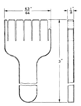
**Feeder brush spacer.** For use in aligning bank feeder brushes, of both the two-piece type and the balanced single-piece type, when remounting 206- and similar-type selectors on the banks.
