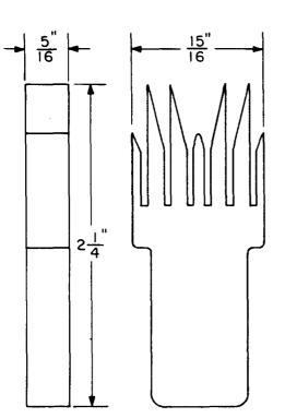
Feeder brush spacer. For use on power driven rotary selectors and 200-, 206-, 209-, and 211-type selectors having six-bank feeder brushes except for those having balanced-type brushes. This tool may be modified for use on selectors having two-or four-bank feeder brushes as covered in Section 026-706-801 and on AECo 25-point rotary switches having one-, two-, or four-bank feeder brushes as covered in Section 026-760-801.
