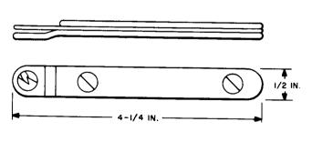
For use in removing outer braid from inside wiring and plastic jacketed switchboard cable. (Specification AT-6691)
