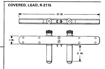
For use in stripping lead-covered cable (PBX installation only).
