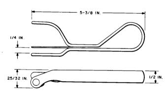
For use in stripping sheath from plastic jacketed switchboard and inside wiring cable.
