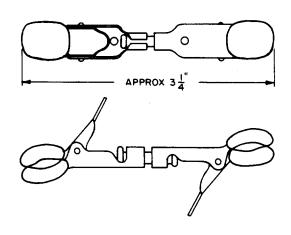
Cord support. This tool forms part of the J94724 contact closure test set. For use with the 587A tool.
