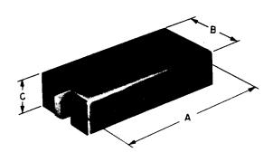
Protector spring supporter. Used on main distributing frames to permit the removal of protector blocks for inspection and cleaning.
