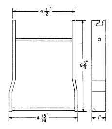
For use on step-by-step type relays and 197- and 198-type switches.
