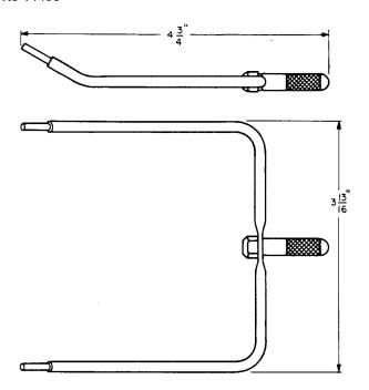
For use in tuning microwave cavities in the TD-2 Radio Systems.
