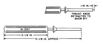
A manually operated wire-unwrapper tool, with an insulated retractable sleeve, used primarily to unwrap and remove solderless-wrapped connections of 22-, 24-, and 26-gauge wires. Replaces the KS-16492 L2 wire-unwrapper.
