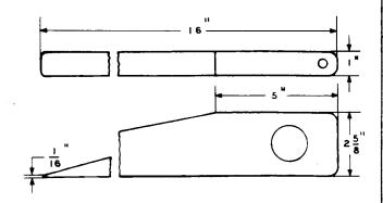
Hardwood wedge. Replaces the 93 tool. For use in lifting multiple cable.
