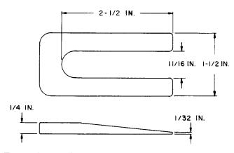
Eccentric coupling wedge. For use on vertical drive shafts.
