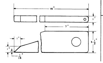
Hardwood wedge. The slanted end of the tool may be cut to any required length. Replaces the 93 tool. For use in lifting multiple cable.
