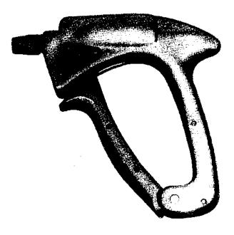
An insulated, hand operated tool which is primarily used for making solderless-wrapped connections on "live" and non-working equipment. This model features a finger-operated chuck which is compatible with the KS-20963 sleeves. Wrapping bits and stationary sleeves must be ordered separately for use with this tool. Refer to Section 074-205-114 for the wrapping bits to be used with this wire-wrapper. Refer to Section 074-256-141 for wrapping sleeves to be used with this wire-wrapper.
