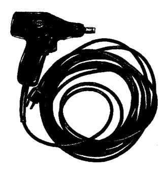
The KS-21232 L1 (electric) wire wrapping gun is used for 20-gauge through 30-gauge wire. It is a lightweight pistol shaped, double insulated, 115-volt ac powered gun with a 20-foot cord. A low transient voltage output permits its use on or near "live" equipment, including ESS. Bits and sleeves currently standardized for 22-, 24- and 26-gauge wire may be used in this gun. Bits and sleeves for 28- and 30-gauge wire are available commercially as indicated below:
