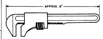
A 9-inch adjustable auto or thin monkey-type wrench. Maximum opening is 2-5/8 inches. Replaces the No. 9, Model G, Billings and Spencer wrench. For use on AMA KS-13928 cleaning cabinet.
