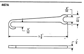
A 9/32-inch open double-end flat wrench. For use on clutch adjusting nuts.
