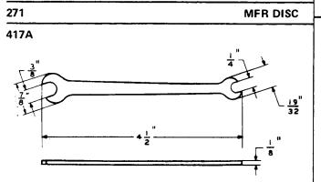
A 1/4-inch and 3/8-inch open double-end flat wrench. Replaces the 244 and 306 tools and the 1/4-inch and 3/8-inch ends of AECO H-7062, H-7063, and H-42316 hex. open-end flat wrenches. For general use.
