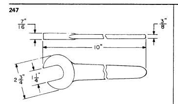
A 1-1/4 inch open single-end flat wrench. For use on friction roll drives, vertical drive shafts, and for general use in power equipment.
