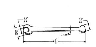
A 25/64-inch flat open-end wrench. For use on the 197- and 198-type switches.
