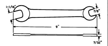
A 7/8-inch and 1-1/16 inch open double-end flat wrench. Replaces the R-2382 wrench. For general use.
