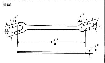
A 5/16-inch and 7/32-inch open double-end flat wrench. Replaces the 7/32-inch and 5/16-inch ends of AECO H-7062 and H-7063 hex. open-end flat wrenches. For general use.
