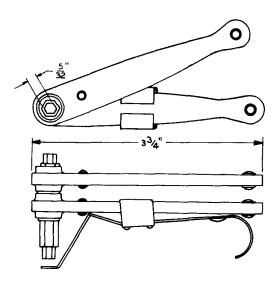
Ratchet Wrench for 5/32-Inch Socket-Head Screws. Replaces the D-176940 tool. For use on the KS-13882 perforators.
