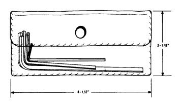
This kit consists of a plastic envelope containing one each of the following sizes of hexagonal socket keys. The keys are for use in turning hexagonal socket set screws and hexagonal socket head cap screws.
