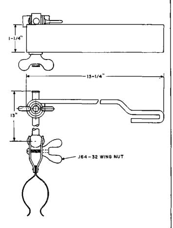
Designed to hook over the top angle of step-by-step switch shelves. The bracket has an adjustable arm for holding a portable lamp guard in various positions.
