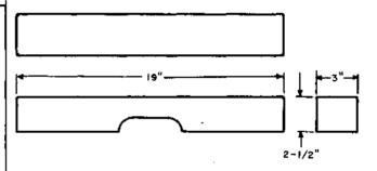
For use in splicing unperforated AMA tape in central offices arranged for AMA.
