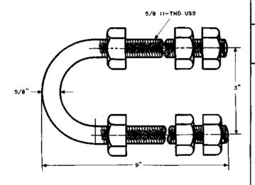
For use in supporting chain hoists from superstructures.
