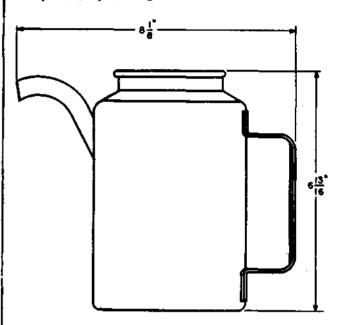
For use in filling KS-16297L1 Flushing Unit with fluid for cleaning and treating bank contacts of Step-by-Step switches.
