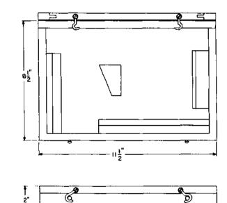
A gray finished wooden case with a hinged cover held closed by a latch. Part of the No. 1014A tool kit and used for housing the tools of that kit. CASE, CARRYING, KS-5672 (specify list No.)
