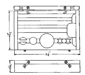
A black finished wooden case with a hinge cover held closed by a latch. Part of the No. 1000A tool kit and used for housing the tools of that kit.
