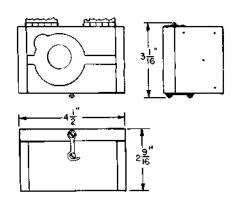
A black finished wooden case with a hinged cover held closed by a latch.
