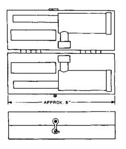
A black finished wooden case with a hinged cover held closed by a latch. Fart of the No. 1003A tool kit and used for housing the tools of that kit. CASE, CARRYING, NO. 19A
