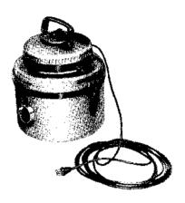
Portable upright tank-type vacuum cleaner for use where heavy duty or silent type, such as KS-14377, is not required. It is approximately 11 inches in diameter and 13 inches high, exclusive of handle. Weight, without attachments, is approximately 17 lbs. It may be mounted on a rolling ladder by using a 32B ladder bracket. It is equipped with a 3-wire 19-foot long KS-14410 L31 power cord.
