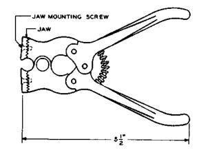
These tools are the same except for the cutting jaws. The jaws (pair) and the jaw mounting screws may be ordered separately when desired. In ordering specify "( ) for (KS- ) cut-nippers".
