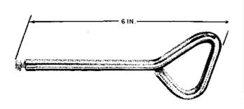
For use in removing packaged semiconductor amplifiers from L-type multiplex equipment.
