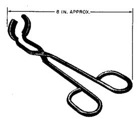
For use in extracting the 375A and similar-type octal base electron tubes and for removing and replacing 89-type resistors.
