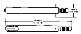
For use in extraction and insertion of 51A pads in L4 Coaxial System.
