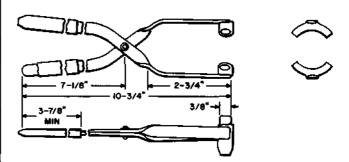
For use in extracting 373A and 374A electron tubes from K2 carrier telephone equipment panels.
