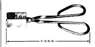
For use in removing the 372A and similar-type patching plugs from the A2A Video System.
