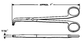
For use in removing and replacing pins in KS-13882 perforators in AMA accounting centers and central offices.
