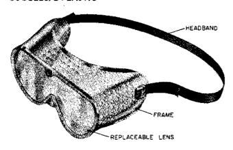
These goggles can be worn over spectacles. The lenses are impact resistant, the frames are ventilated and the headband is adjustable.
