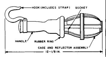
Consists of a soft rubber handle with a fiber guard, a lamp socket and a hook.
