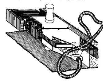
Consists of four 110-volt, 1 amp heating units assembled to a holder. Furnished with a 25-foot heater cord and a switch for closing and opening circuit to heating units. For flat tubes in keyboards where space is limited.
