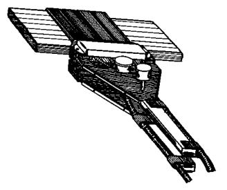
Consists of four 110-volt, 1 amp heating units assembled to a holder. Furnished with a 25-foot heater cord and a switch for closing and opening circuit to heating units. For flat tubes where space is not limited.
