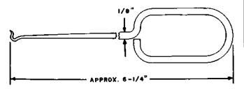
For use in attaching selector elevator apparatus trip rod rotating lever retractile springs and on No. 1A regenerator units.
