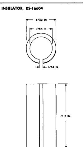
A phenol fiber insulator intended for use on the 121-type Central Office protector to prevent accidental contacts on the cross connecting terminals.
