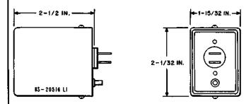
A metal enclosed, single-unit device consisting of a relay driven by a transistorized, astable multivibrator which is powered by a 4 volt dc source.
