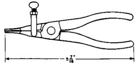
For use in installing internal snap-rings in 1-type translators.
