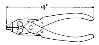
For use in replacing the terminals of the KS-14173 jacks in the N1 Carrier Systems.
