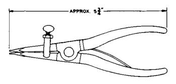
For use in installing external snap-rings on motor mounting shafts in KS-13834 perforator.
