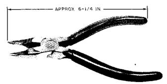
The B and C short-nose pliers (Spec. AT-8479) are identical except that the jaws of the C pliers are coated with aluminum oxide for electrical insulation. Both are equipped with orange plastic cushion grips.
