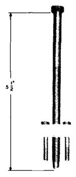
For use with Owatonna Tool Co. No. 950 Bearing Pulling Attachment to remove ball bearing race from shaft of blower motor used in the KS-16001 Dehydrator. PULLER, ROTOR, K3-5331
