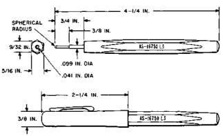
Consists of a metal pin mounted in a cast resin handle and a removable cap.
