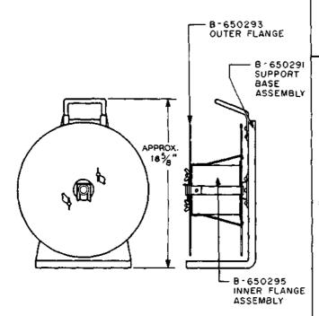
For use in central offices for holding distributing frame wire.
