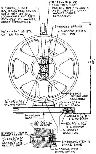
For use in central offices for holding distributing frame wire.
