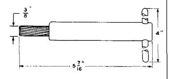
For use with the D-97086 guide and clamp nut, for reaming housing assembly bearings of friction roll drives to relieve overheating.
