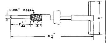
For use with the D-97084 tapered bushing in reaming bearings in worm case housings of friction roll drives to relieve overheating.
