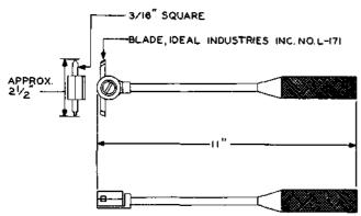
For use on generator and motor commutators and on interrupter drums.
