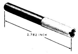
L2 sleeve (coded red) is intended for use with a 22-24 gauge combination bit.
