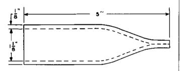
Electron tube shield For use on 430A vacuum tubes in AMA Systems.
