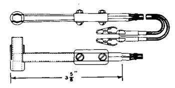
Consists of a 38A lamp socket equipped with an M2CP cord (6' 6"). Intended for use with a 2-type switchboard lamp. The 2-type lamp must be ordered separately.
