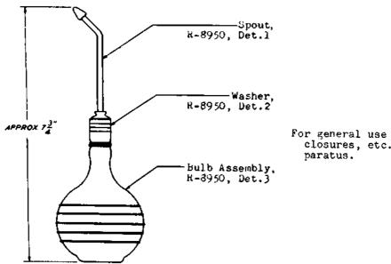
For general use in flushing bearings, oil closures, etc. of various kinds of apparatus.
