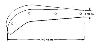
For use in cleaning plunger-type line switch springs.
