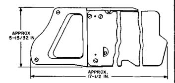
For use in bulk handling of 200 blanks and coded cards when servicing 1-type translators.
