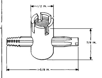
For pressure testing purposes, (Spec. AT-7471X)
